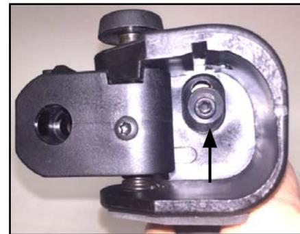
5 Using the appropriate allen wrench, secure the buttstock to the receiver by tightening the bolt as seen in Figure 5.
