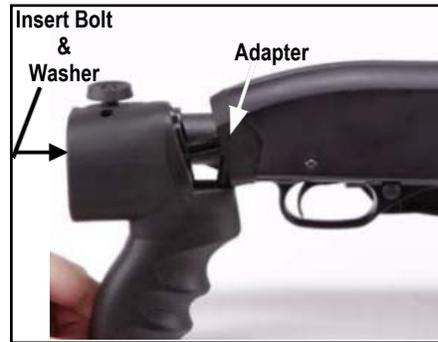
4 With the buttstock in the folded position, place the appropriate bolt with the supplied washer through the rear of the pivot housing and the appropriate adapter as seen in Figure 4.
