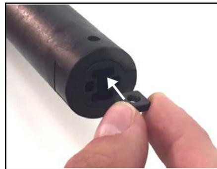
6 Take the buffer tube and turn over and install the provided 8-32 square nut into the buffer top hole tube as seen in Figure 6. NOTE: The screw in the step 8 will tighten into this square nut.
