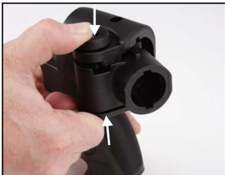
3 Next, put your stock into the folded position by pressing together on the pin cap and under the pivot housing as seen in Figure 3.
