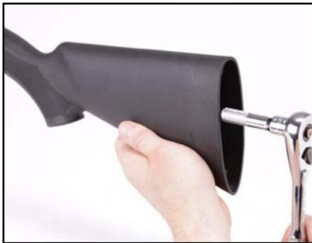
1 Begin by removing the existing recoil pad from your stock using a phillips head screwdriver. Next using a long flat head screwdriver or the appropriate socket with extension remove the stock bolt from the inside of the opening in the rear of the stock as seen in Figure 1.
