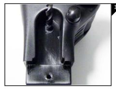
If the screw measures .230 remove the pivot assembly and start by drilling pilot holes in the center of the 2 marked holes with a 1/16" starter drill bit as seen in Figure 3. Next, move up to the 3/16" drill bit and drill 2 wider holes using the two pilot holes.
