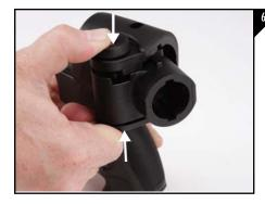
Next, put your stock into the folded position by pressing together on the pin cap and under the pivot housing as seen in Figure 6.
