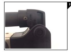
Using the provided 8-32 x 5/8" Button Head Cap Screw and a 3/32 allen wrench, tighten the buffer tube to the pivot housing as seen in Figure 8.
