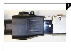
After disassebling your AK using your owners manual, begin by placing the pivot housing assembly into the receiver as seen in Figure 1
