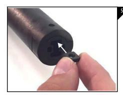
Turn the tube over and install the provided 8-32 square nut into the top hole on the tube as seen in Figure 5.
