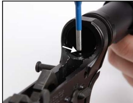
4 Using a punch, depress the buffer retainer pin as seen in Figure 4 and begin to unscrew the existing buffer tube.
