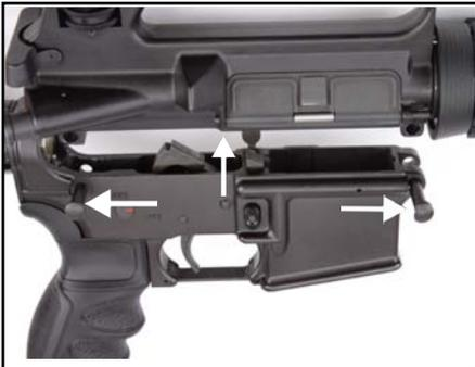
1 Begin by depressing and removing the front and rear take down pins and then detaching the lower and upper receiver as seen in Figure 1.
