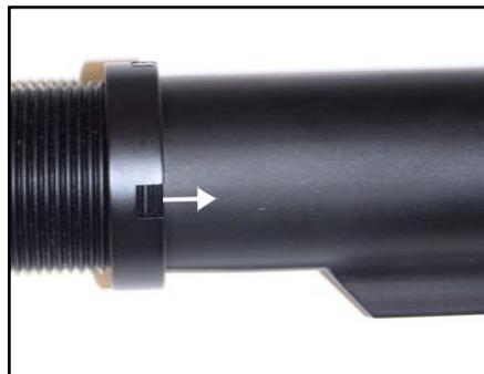
6 Install the new buffer tube by screwing on the castle nut, making sure the teeth are facing to the rear of the weapon as seen in Figure 6.
