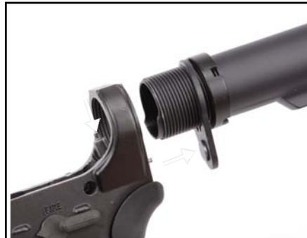
5 Once the tube clears the buffer retainer pin you may then finish unscrewing and remove the buffer tube leaving the pin in place as seen in Figure 5.
