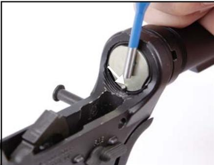
2 Using a punch, depress the buffer retainer spring as seen in Figure 2 and then remove the spring. When removing the spring be careful as the spring is under heavy tension.
