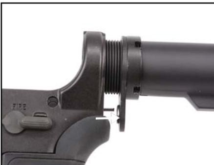
3 Next, using an AR tool, loosen the existing castle nut and slide the locking ring to the rear as seen in Figure 3. When sliding the locking ring keep in mind that the spring for the rear take down pin is under tension.
