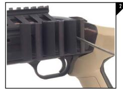
Next, using the provided 10-32 x 1/4" Low Profile Socket Cap Screw and M6 Lock Washer, tighten the Add-a-Shell to the Side Saddle using a 1/8" allen wrench as seen in Figure
