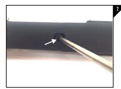
Once the barrel is seated into the ATI stock turn the stock on its side and using a phillips head screwdriver, the provided 1/4" lock washer and the original action mouting screw, tighten as seen in Figure 2.
