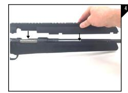
Remove the spring and follower from the old trigger guard/magazine and place the spring inside the mag well with the shell follower face up. Next install the top cover to the stock body as seen in Figure 4.
