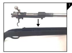
Begin by removing the barreled action from the existing stock. Using a small punch drivout the retaining pin from the rear sight and then tap the spring toward the front sight and lift out the rear sight. Place the barreled action into the ATI Mauser stock as seen in Figure 1.
