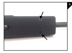
Turn your firearm over and using a phillips head screwdriver and the provided (2) #8 x 2" sheet metal screws tighten the stock body to the top cover as seen in Figure 6.
