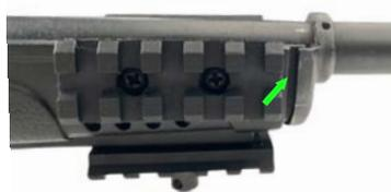
Next, install the barreled action into the stock body, making sure the stock is as far forward on the action as it will go and slide into place as seen in (Figure 8a). You will also want to make sure the front of the stock body seats into the band on the front of the barreled as seen in (Figure 8b).
