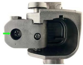
With the knuckle in the folded position, slide the buffer tube into the knuckle as seen in (Figure 13a). Using a Phillips Head Screwdriver and the provided 14 x 1 1/4" Phillips Head Screw (#1), tighten the tube through the back of the knuckle as seen in (Figure 13b).
