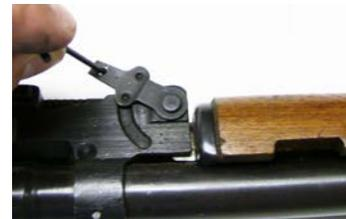
Using a punch or small screwdriver, raise the lever on the right side of the rear sight base as seen in (Figure 3a). The dimple on the lever should stop at the end of the curved track on the right side of the rear sight base..
