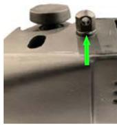
To install the top sling stud (# 9), locate the hole on the top of the stock near the folding button as seen in (Figure 4a). Using an adjustable wrench, tighten the sling stud until seated as seen in (Figure 4b).
