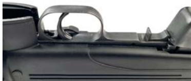
To install the trigger assembly, insert the front of assembly into the stock making sure the cross pins go to locator lugs on the bottom of the receiver as seen in (Figure 9a). Tap the trigger guard forward and firmly push down on trigger assembly until it locks into place as seen in (Figure 9b).
