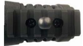
Next, install (2) 6-32 hex nuts (#7) into the pockets on the bottom of the inside stock body as seen in (Figure 6c). Align the bottom rail into place and while holding a finger over the hex nuts, fasten the rail using (2) 6-32 x 3/8" machine screws (#5) and a phillips head screwdriver as seen in (Figure 6d).
