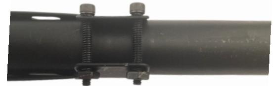
Depending on the size of your barrel, using a 7/64" allen wrench you will now use the (2) provided 6-32 x 3/4" or 6-32 x 1" screws (# 1 or #2) and the provided 6-32 hex nuts (#4) and tighten the heat shield to the barrel as seen in (Figure 3d & 3e).
