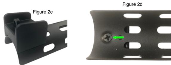
Once the rear sight is seated on the heat shield as seen in (Figure 2c), flip the heat shield over and while holding onto the sight tighten the sight using one of the provided #6 x 3/8" screw (#3) as seen in (Figure 2d).
