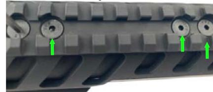
For installation on a Mossberg, using the provided (4) 8-40 x 3/8" flat head screws (#2) and a 3/32" allen wrench as seen in (Figure 1d) tighten the side saddle until snug as seen in (Figure 1e). For installation of the side saddle on a Winchester or Remington use the provided (4) 8-32 x 3/8 flat head screws (#3) and a 3/32" allen wrench.
