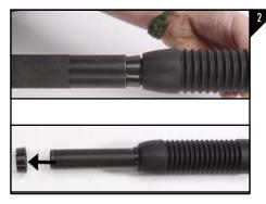
Using the appropriate magazine socket wrench or spanner wrench, unscrew the forend nut and than remove the nut and forend as seen in Figure 2.
