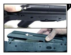
Begin by pressing in the button on the rear of the receiver cover. Next remove the cover from the slot in the rear of the sight housing and set aside as seen in Figure 1.
