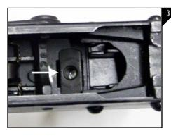
Locate the pistol grip nut on the inside of the receiver as seen in Figure
