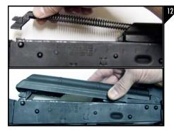
Reinstall the rod and spring into the bolt carrier and the place the rear end of the rod into the slot in the rear of the receiver. Next reinstall the receiver cover by placing the front of the cover into the slot in the rear sight housing and then locking into place with the rear end of the rod through the cover as seen in Figure 12.
