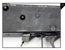
If the psitol grip nut comes out of place, position the T-nut as shown below as seen in Figure 7.
