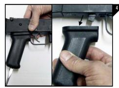
While holding the pistol grip nut, remove the screw from the bottom of the pistol grip using a flat head screwdriver or allen wrench and then remove the grip as seen in Figure
