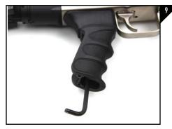
Continue to hold the T-nut and pistol grip in place. Using a 5mm allen wrench, completely thread the M6 X 1 x 25mm Socket Head Cap Bolt into the T-nut, and secure the ATI psitol grip ot the AK-47 receiver as seen in Figure 9.
