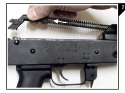
Push the rear of the rod towards the barrel until it is free from the receiver and then pull the rod up and back to remove the rod and spring from the bolt carrier as seen in Figure 2.
