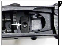
Locate the pistol grip T-nut on the inside of the receiver as seen in Figure
