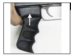
While holding the pistol grip nut, slide the new ATI AK-7 Pistol grip over the nut as seen in Figure 8.
