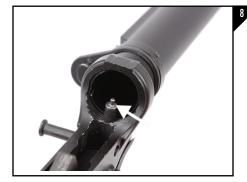
Next, screw the buffer tube into the lower receiver until you come in contact with the buffer retainer pin and the buffer tube stops as seen in Figure 8.
