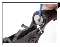
Reinstall the buffer and spring into the buffer tube until the spring is seated behind the buffer retainer pin as seen in Figure 12.
