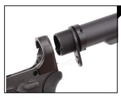
Once the tube clears the buffer retainer pin you may than finish unscrewing and remove the buffer tube leaving the pin in place as seen in Figure 5.
