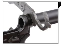
Hand tighten the castle nut to hold the locking ring in place, then take the AR tool and tighten the castle nut until tight as seen in Figure 11.
