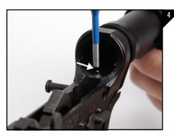
Using a punch, depress the buffer retainer pin as seen in Figure 4 and begin to unscrew the existing buffer tube.
