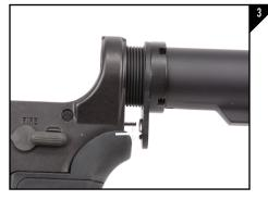
Next, using an AR tool, loosen the existing castle nut and slide the locking ring to the rear as seen in Figure 3. When sliding the lockng ring keep in mind that the spring for the rear take down pin is under tension.
