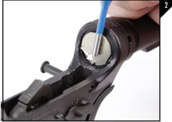
Using a punch, depress the buffer retainer spring as seen in Figure 2 and than remove the sring. When removing the spring be careful as the spring is under heavy tension.
