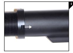
Install the new buffer tube by screwing on the castle nut, making sure the teeth are facing to the rear of the weapon as seen in Figure 6.
