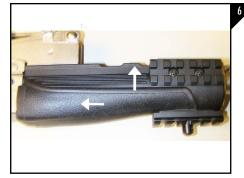
The lower handguard should be positioned with the ribs on the front sight housing and the end of the handguard in front of the receiever. Push up, then slide back onto the receiver as seen in Figure
