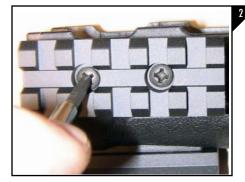
Using the provided 6-32 x 1/2" machine screws and a phillips head screw driver tighten the rails to the handguard as seen in Figure 2.
