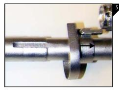
Unlock the front mounting bracket lever and slide the mount bracket down the barrel as seen in Figure 5.
