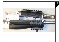
Install the gas tube into the gas piston. Next, align the upper handguard with the lower handguard and press the rear of the gas tube down until the lever can be locked as seen in Figure 9.
