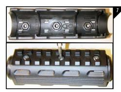
If you choose to install the 4" picatinny rail on the upper handguard, place the rail onto the slot then place the supplied 6-32 hex nuts in the nut pockets on the inside of the handguard. Next install the 6-32 x 5/16" supplied machine screws and tighten until snug as seen in Figure 7.
