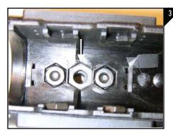
If desired, install the bottom swivel stud by placing the supplied 10-32 hex nut into the proper location as seen in Figure
