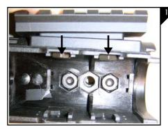
If you choose to install the 2" rails on the bottom and or sides of the lower handquard begin by placing the rail onto the hanguard. Next place the supplied 6-32 hex nuts into the pockets on the handguard as seen in Figure 1.
