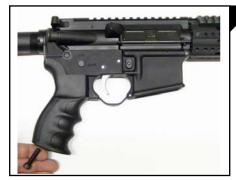
Insert the grip bolt through the bottom of the grip and tighten using a 3/16" standard allen wrench as seen in Figure 4.
