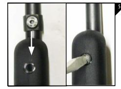
Align the barrel band with the hole in the forearm and use the original forearm screw to fasten the front of the forearm to the barrel band as seen in Figure 5.
