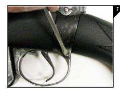
Align the original trigger guard rear screw with the trigger guard screw hole. Begin to thread the screw in place but do not tighten all the way as seen in Figure 7.
