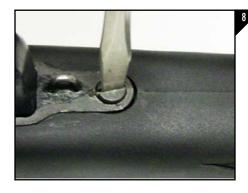
Insert the original trigger guard front screw and using a flat head screwdriver, completely tighten the screw as seen in Figure 8. Once the front screw is fastened, you can now go back and completely fasten the rear trigger guard screw.
