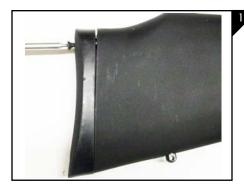
Using a phillips head screwdriver, remove the butt pad from the new ATI Monte Carlo Stock as seen in Figure 1.
