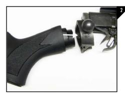
Install the new buttstock using the original rear attaching stock bolt. Tighten the bolt, and secure the new buttstock to the rifle as seen in Figure 2.
