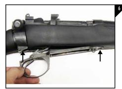
Next, align the trigger guard back into the place so the trigger is properly engaged with the sear as seen in Figure 6.
