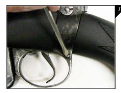
Align the original trigger guard rear screw with the trigger guard screw hole. Begin to thread the screw in place but do not tighten all the way as seen in Figure 7.
