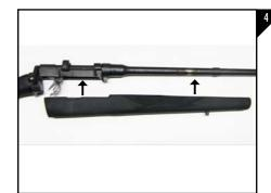
Lay the rifle on a work bench or a table and work the new ATI Monte Carlo forearm over the barreled action as seen in Figure 4. Do not fasten the forearm at this point.
