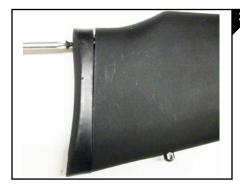
Next, using a phillips head screwdriver and the screws removed in Figure 1, reinstall the butt pad to the rear of the buttstock as seen in Figure 3.
