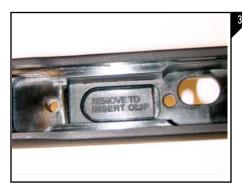
For clip fed rifles, remove the oval recessed area in the bottom of the stock, just forward of the trigger assembly opening as seen in Fiugre 4. Stock material is easily removed with most common woodworking tools, drills and files.
