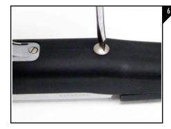
Install and tighten the take down screw that was removed in step 1 using flat head screwdriver as seen in Figure 6.
