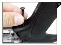
Install the provided 8/32 x 2" screw through the trigger assembly. Because this screw passes through the hole in the rear of the trigger assembly, it may be necessary to loosen the front screw of the trigger assembly. Tighten with a phillips head screwdriver until snug as seen in Figure 8.
