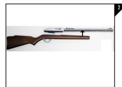
Next, lift the barreled action out of the old stock as seen in Figure 2.
