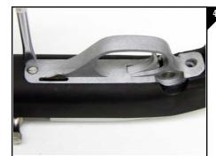
Install the trigger assembly into the ATI Fiberfoce (the snug fit is intentional) and reinstall the flange nut and trigger retaining screw that was removed in step 3 as seen in Figure 4.
