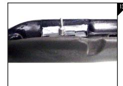
Use a dremel or similar tool to remove material from the stock wall as seen in Figure
