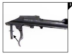
Once you have determined that a washer will be needed for the proper fit, disassemble the firearm. Place the top receiver screws through the receiver and then slide the 5/16" washer provided onto the end of the bolt as seen in Figure 8.
