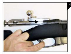
Reinstall the bolt by depressing the trigger and pusing the bolt forward into the barreled action as seen in Figure 4.
