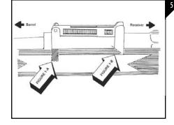
For modifications for rear sight clearance on the M-39 Finnish Heavy Barrel, material must be removed from the shaded area as seen in Figure 5. Cut a slot approx. 1/16" x 5/16 wide x 3/8" deep on both the front left and front right sides of the stock indicated by arrow 1-A. This may be best accomplished using a dremel tool. To obtain the correct rear clearance. simply file approx. 1/8" off of the corner as indicated by arrow 1-B.
