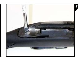
Turn the rifle over install and tighten the top receiver screw as seen in Figure 11. NOTE: When the washer is installed, there might be a small gap between the barrel and the stock. This will not affect the performance of the firearm.
