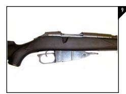
Next, insert the barreled action with the bolt and washer into the top of the stock and insert the magazine assembly into the bottom of the stock as seen in Figure 9.
