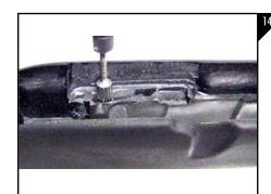
The side wall of the stock gets thicker as it moves down the side. Be sure to angle the dremel so the wall had the same thickness on the top as it does on the bottom as seen in Figure 14.
