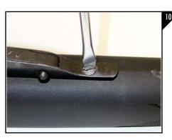
Using a flathead screwdriver install and tighten the bottom magazine screw as seen in Figure 10.
