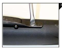
Next, using a flathead screwdriver install and tighten the bottom magazine screw as seen in Figure 2.
