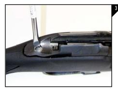
Turn the rifle over install and tighten the top receiver screw as seen in Figure 3.
