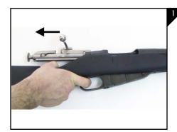
Begin by removing the bolt assembly from the action by squeezing the trigger and pulling out towards the rear as seen in Figure 1.
