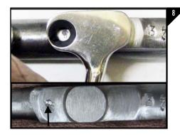
Mark the hole location, then using the (larger) #11 drill bit, carefully spot drill for the mounting screw, just deep enough to create a centered starting point as seen in Figure 8.
