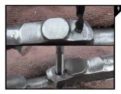
Using the supplied #21 (smaller) drill bit, drill through the center of the bolt forging. While still clamped, use the 10-32 tap and tap the hole drilled into the bolt as seen in Figure 9. Deburr and throughly clean the bolt and handle.
