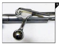
Place the ATI bolt handle in place on the bolt and install and tighten the supplied 10-32 countersunk machine screw as seen in Figure
