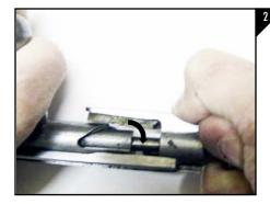
To disassemble the bolt, grasp the bolt handle, pull rearward and turn the cocking piece1/4 turn to the left, making sure the bolt guide bar remains intact as seen in Figure 2.
