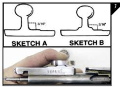
For "non-stepped" (sketch A) press the 1/2" spacer inside the ATI bolt handle. If "stepped" (sketch B) the bolt handle does NOT require a spacer. Place the ATI bolt handle over the knob on the orginal bolt as seen in Figure 7.
