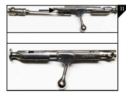
To assemble the bolt, place the bolt and bolt guide bar back on the bolt assembly. Grasp the bolt handle, pull rearward and turn the cocking piece 1/4 turn to the right as seen in Figure 11, making sure the bolt guide bar remains intact and lined up with the bolt assembly.
