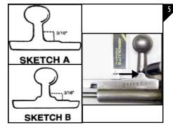
Mark the bolt handle base with a marker and measure upward 3/16" on the knob shank from the base of the bolt and scribe a line as seen in Figure 5.
