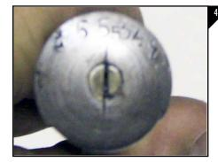
Note the position marks at the rear of the bolt as seen in Figure 4. This aligns the firing pin depth correctly and must be returned to exactly the same position for safe operation.
