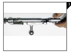
The bolt head and guide bar slide will remove by sliding them forward off the bolt assembly, exposing the firing pin as seen in Figure 3.
