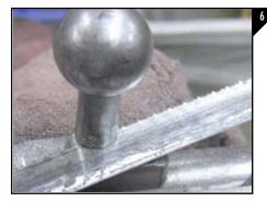
Clamp the bolt in a padded vise with the bolt handle upward. Re-check the 3/16" measurement, leaving room for finish filing. Next, cut off bolt handle as seen in Figure
