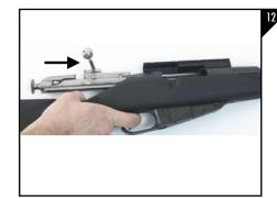
Install the bolt assembly by squeezing the trigger and pushing the bolt into the chamber as seen in Figure 12
