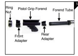
After removing the plastic bridges, assemble the forend to all models as shown. Due to varying receiver widths there may be interference between the rear of the forend and the front of the receiver. If it occurs use a rotary tool or file to remove material from the rear of the forend. To reassemble your firearm reverse steps 1-4.
