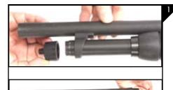
Begin by unscrewing the magazine cap by turning the cap counter clockwise and then removing the barrel by pulling it out of the receiver as seen in Figure 1.
