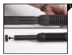
Using the appropriate magazine socket wrench or spanner wrench, unscrew the forend nut and remove as seen in Figure 2.
