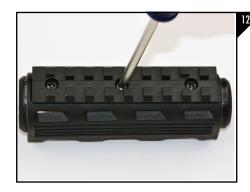
If you choose to install the 4" picatinny rail on the upper handguard, place the rail onto the slot then place the supplied 6-32 hex nuts in the nut pockets on the inside of the handguard. Next install the 6-32 x 5/16" supplied machine screws and tighten until snug as seen in Figure 12.
