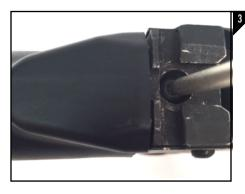
Before proceeding make sure you remove the mount from the reciever. Using a 5/32" drill bit, drill through the marked hole about 1/2". Place the mount into the receiver of the AK-47 and using the provided 8 x 48-2 x 1/2" plastite pan head torx screw tighten the mount to the receiver as seen in Figure 3.
