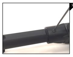
Flip your AK over and using the provided 8-32 x 5/16" button head cap screw and a 3/32 allen wrench tighten the buffer tube to the mount as seen in Figure 5.
