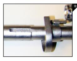
Unlock the front mounting bracket lever and slide the mount bracket down the barrel as seen in Figure 10.
