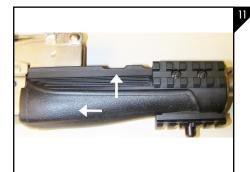
The lower handguard should be positioned with the ribs on the front sight housing and the end of the handguard in front of the receiever. Push up, then slide back onto the receiver as seen in Figure 11.
