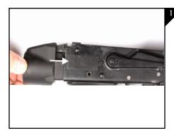
After disassebling your AK using your owners manual, begin by placing the elite mount into the receiver as seen in Figure 1.
