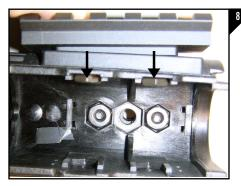
If you choose to install the 2" rails on the bottom and or sides of the lower handguard begin by placing the rail onto the hanguard. Next place the supplied 6-32 hex nuts into the pockets on the handguard as seen in Figure 8.
