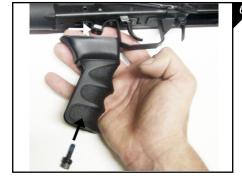
Install the new ATI pistol grip by holding the supplied pistol grip T-nut onto the pistol grip mount bracket (shown with small red arrow below). Now, slide the pistol grip and the M6 x 1 x 25mm into place behind the trigger guard. Use a 5mm allen wrench to fasten the pistol grip bolt to the pistol grip nut on the mount bracket as seen in Figure 6.
